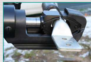
Open crimping head and handle facilitates positioning
