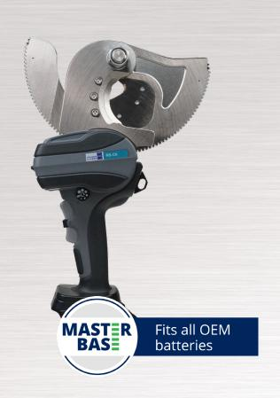
The overhead line cutter quickly and powerful cuts ACSR up to Ø 54 mm with steel part up to 70 mm<sup>2</sup>, such as 550/70. In overhead line construction this lightweight and ergonomic tool convinces with its cutting pattern and high efficiency thanks to well matched drive unit.
