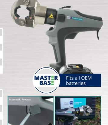
This powerful battery-hydraulic crimping tool processes cable lugs and connectors up to 400 mm<sup>2</sup> according to DIN with standard C-shaped crimping dies, even wide crimps facilitate the crimping process. Its versatility makes it suitable for use in power supply companies, municipal utilities, industrial cable assembly or wind energy.
