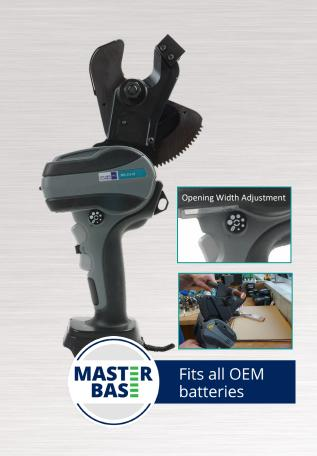
The battery-operated cutting tool with its open cutting geometry cuts copper and aluminium strands and power cables up to  $\emptyset$  33 mm, round material as well as ACSR up to  $\emptyset$  18.6 mm (max. steel content 35 mm<sup>2</sup>).
