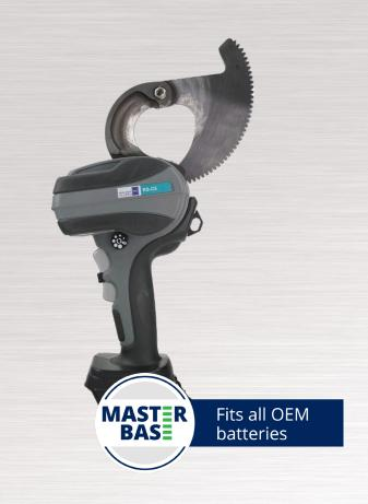
The cable cutter precisely and quickly cuts Cu and Al cables up to  $\emptyset$  50 mm, such as NAYY 4 x 185 mm<sup>2</sup> and Cu single cores up to 630 mm<sup>2</sup>. In power supply and cable processing, this lightweight and ergonomic tool convinces with its sickle-shaped cutting geometry.
