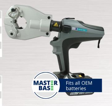
The battery-hydraulic crimping tool crimps with a self-centering, integrated 4-arbor system non-insulated, fine-stranded Cu conductors according to DIN 60228, class 2, 5 and 6 in ranges 16 - 300 mm<sup>2</sup> and is used in switch gear construction as well as for aggregate connections. No crimping dies are required.
